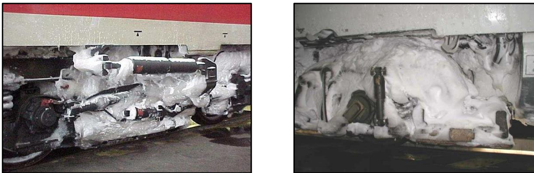
(a) (b) Figure 5. (a-b) Wet-snow accretions on bogies train [18].
