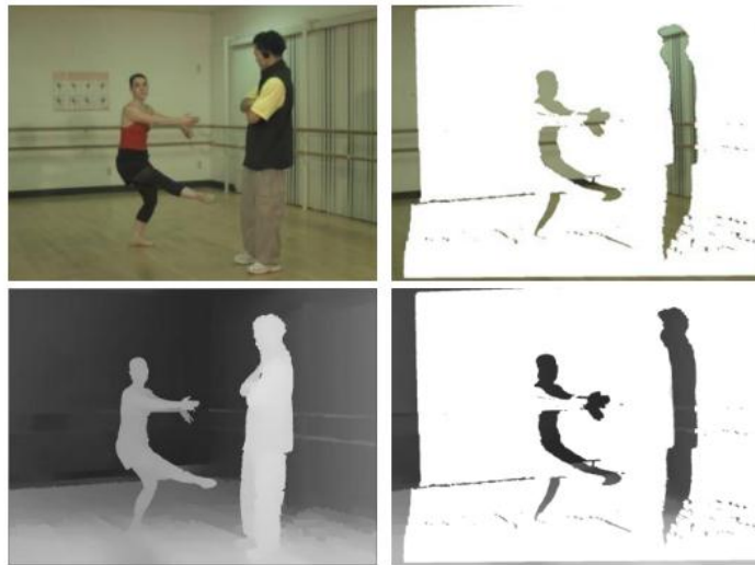
Figure 1-14 : LDV format: color (top) and depth (bottom) of main layer (left), occlusion layer (right) (Fig. 5-1, page 52 from (Kerbioui et al., 2010))
