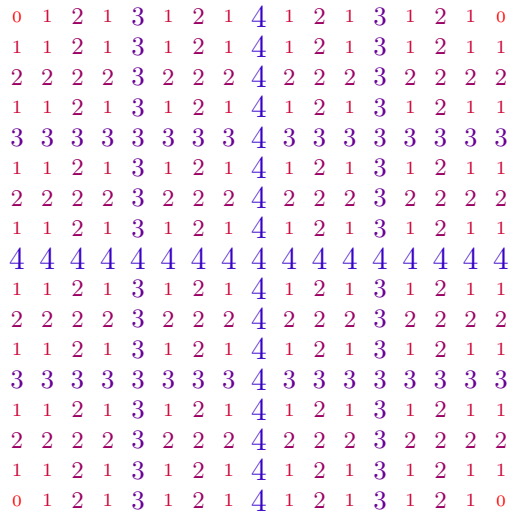
Figure 8.2: Level sets of separators for n = 16 . Nodes with the same number k belong to the same set of separators Sep_k . Each set of separators Sep_k consists of several “+”-shaped separators.
