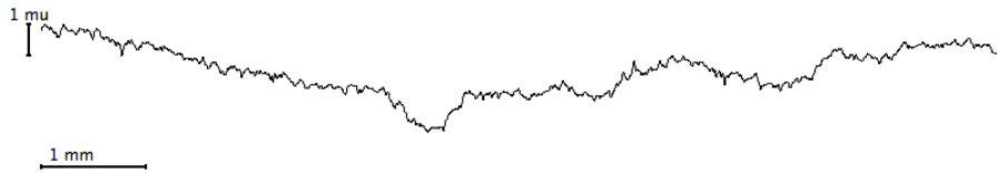
Figure 2.22: Typical example of surface profile of CNPRE 1% composite
