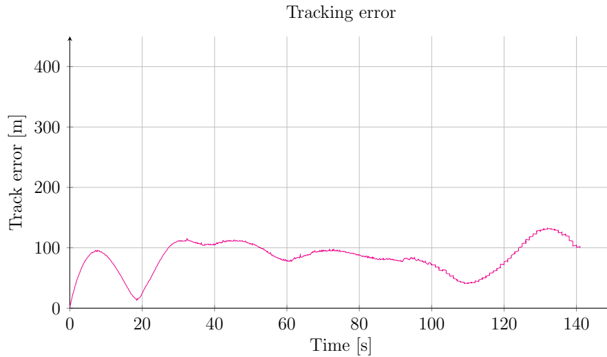
FIGURE 5.24: Tracking error (flight experiments with Pilatos 3).
