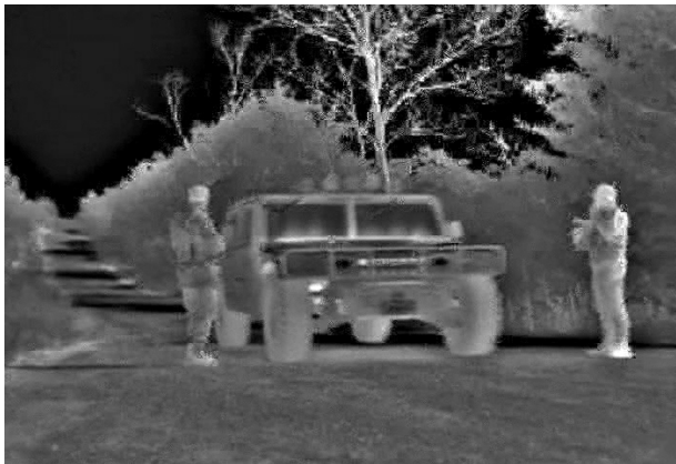
(b) Reconstruction OMP, SNR_{rec} = 16.2 dB
