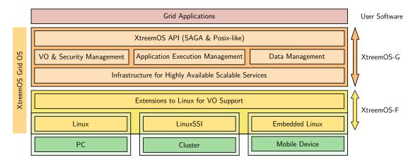
Figure 2.5: Overview of XTREEMOS's architecture
