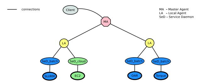
Figure 2.7: Overview of DIET's architecture when used as a meta-scheduler
