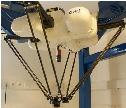
Figure 2.7 – The Quattro parallel robot with a base-mounted camera ( left ) and its joint-oriented graphical layout ( right ).
