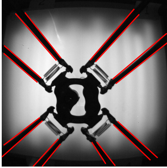
Figure 4.2 – The 16 edges (red lines) from 8 cylindrical legs of the Quattro robot for a given pose in calibration.
