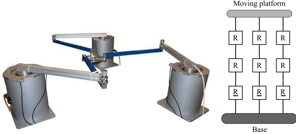
Figure A.5 – The 3-RRR planar parallel robot ( left ) and its graphical layout ( right ).
