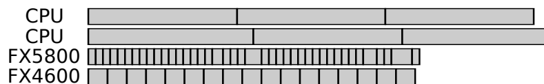
Figure 3.1: A pathological case: Gantt diagram of a blocked matrix multiplication with a greedy scheduling strategy.
