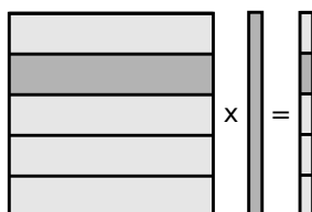
Figure 2.5: Example of a matrix-vector product using data filters: the input matrix and the output vector are partitioned in five sub-parts which can be computed independently. The data accessed to compute the second sub-vector are for instance shown in dark.
