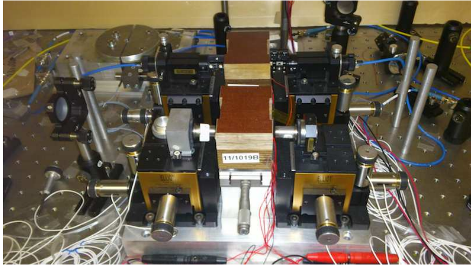
Figure 3.20.: Picture of the experimental setup for wavelength conversion. The two PPLN/Ws are enclosed in temperature stabilized ovens made of Bakelite (brown material). The waveguide in the front is free-space coupled at the in and output using aspheric lenses. The waveguide in the background is in the final configuration being fibre coupled at the input and output. In the top left corner of the picture, the piezo fibre stretcher is seen (two metallic half circles mounted on a translation stage). On top of the picture the beginning of the polystyrene box is seen (yellow).
