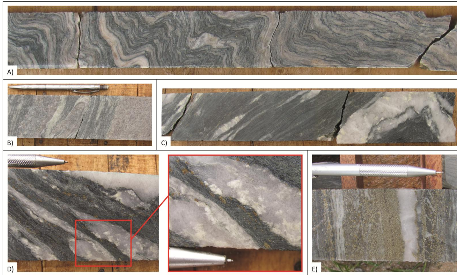
Figure II-11 Examples of mineralisation at the Wassa mine. A) Intensely foliated and mineralised “mafic volcanic” with foliation parallel veins and later folding. Drill hole NSADD006, 157-158m, 1.36 g/t Au. B) Isoclinal F1 folds defined by earlier foliation in contact with porphyry unit. Drill hole SED0027. C) Intensely foliated and mineralized “mafic volcanic” unit and early QV1 veins boundinaged along the foliation, a later stage thicker quartz carbonate vein is located at right hand side of figure (inferred QV4 vein set). Both veins sets are folded. Drill hole NSADD009 214-215m, 3.38 g/t Au. D) Mineralized and boudinaged QV1 veins with adjacent disseminated pyrite. The enlarged section highlights the pyrite is deformed within the S1 foliation and is therefore pre- to syn-D1. Drill hole NSADD009 212-213m 2.48 g/t Au. E) Disseminated pyrite adjacent to QV1 veins. Drill hole BSDD090.
