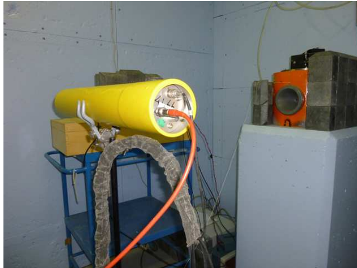
Figure 2.15: Photo of the experimental setup at CoCase. The IC (yellow) is located in front of the CoCase source (orange).
