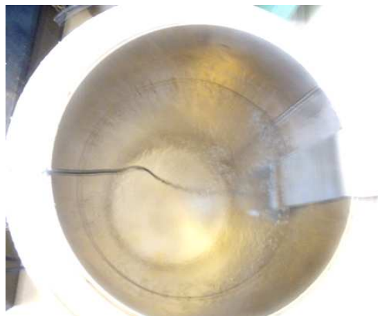
Figure 2.24: Photo of the CVD diamond test in liquid nitrogen with a ^{252}\text{Cf} source outside the Dewar.
