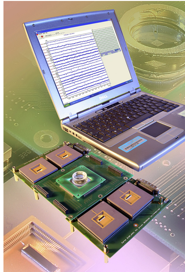
Fig. 3. Picture of the complete BioMEA TM system including a controller (power supply and data acquisition), a MEA holder (ASIC electronics and MEA biochip interface) and a computer user interface.
