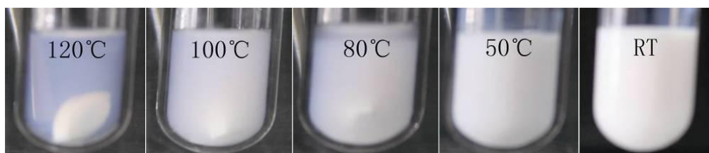
Fig3.13 Optical appearance of E2: St/octane ( v/v ) = 1/2, [St]/[PMAiBuPOSS_{13}] = 2550 , 120°C, 15h at different temperature during cooling
