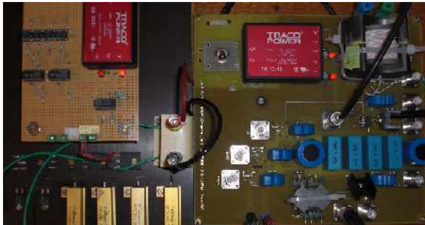
Figure 3.8: SEPIC prototype (right) with load variation kit (left).
