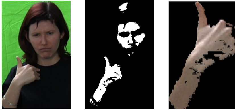
Figure 4.1: Skin segmentation result using an explicitly defined skin model in RGB colour space
