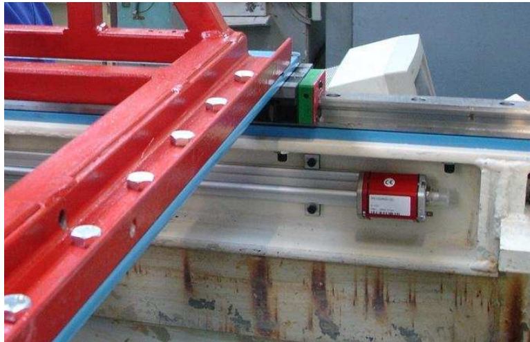
Figure 3.4: Sliding system of a trolley
