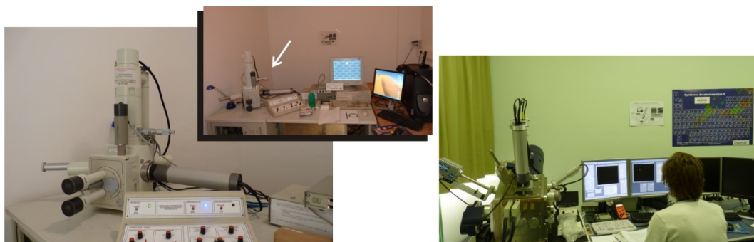
Figure 3-8. JEOL JSM 5600 (left) and CamScan X5000FE CrystalProbe facilities et Geosciences Montpellier (France).
