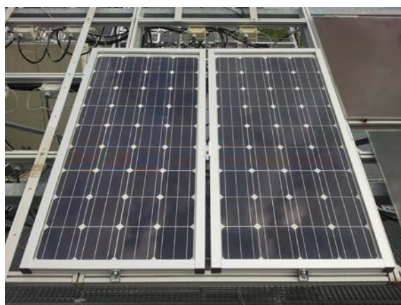
Figure 5.11. PV modules issued from HJ solar cells to be tested at the laboratory and for outdoor operation.
