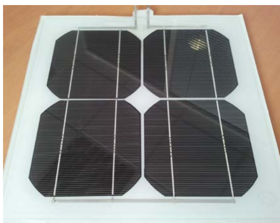
Figure 5.11. PV modules issued from HJ solar cells to be tested at the laboratory and for outdoor operation.
