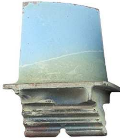
Figure 1.3: Picture of a coloration, technique in which the temperature seen by the blades corresponds to a color scale, courtesy of TURBOMECA.
