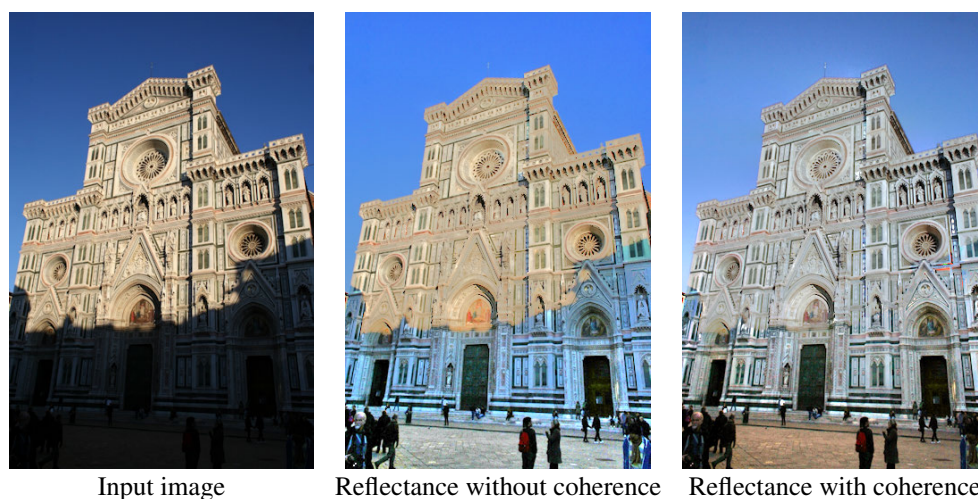
Figure 5.17: Comparison between the decomposition, before and after multi-view coherence in the Florence scene. The coherence constraints between multiple views allow our method to recover a coherent reflectance even under mixed lighting conditions such as this bright sun with blue shadows.
