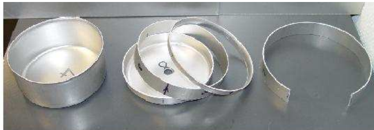
FIGURE 4.1 – From left to right, experimental drawn cup, cut rings and springback after splitting
