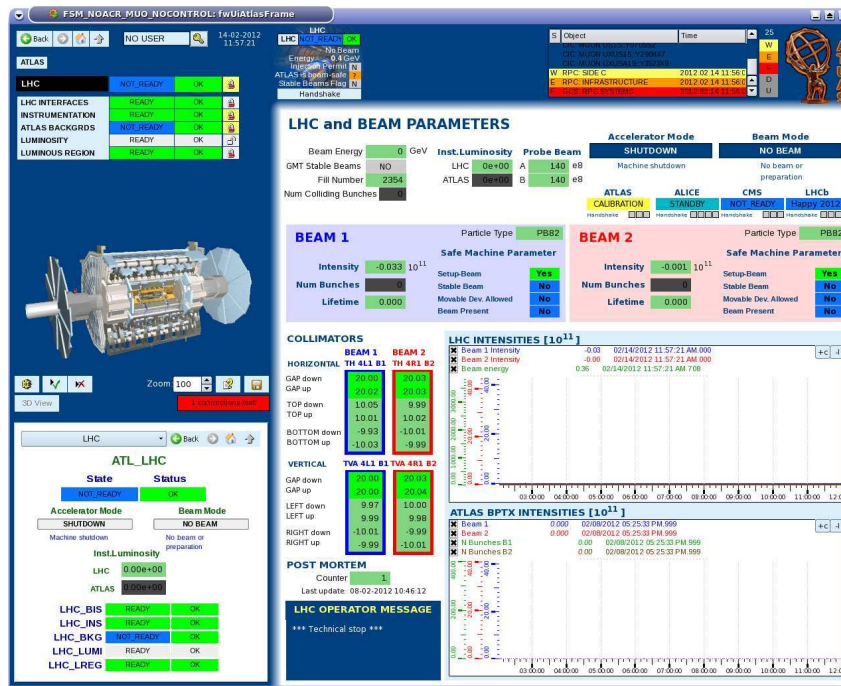
Figure 3.3: The FSM panels are one of the main shifter tools in order to control and monitor the detectors. There are panels for every node of the FSM tree providing the necessary information.
