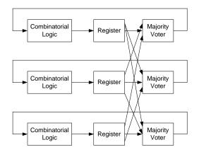
Figure 4.14: Triple modular redundancy with three independent voters [27].
