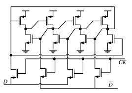
Figure 4.13: Schematic diagram of DICE [30].
