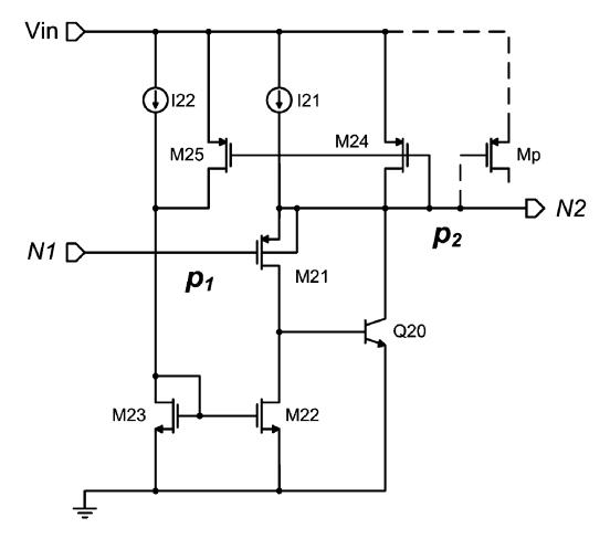
Figure 5.5: Buffer with dynamically-biased shunt feedback [17].
