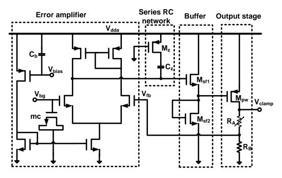
Figure 5.9: Schematic diagram of the RegVclamp.
