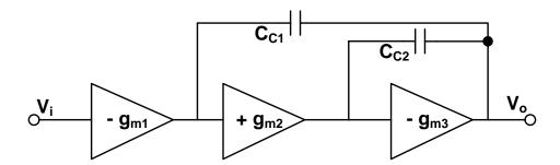
Figure 5.3: A three-stage amplifier with nested Miller compensation.
