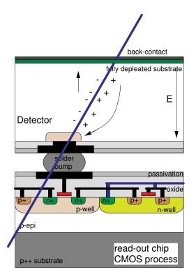
Figure 1.8: The architecture of hybrid pixel sensor [8].
