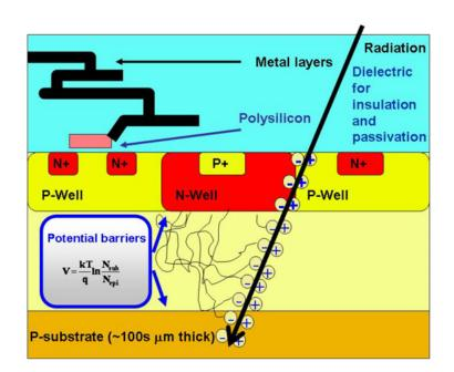
Figure 1.10: Schematic cross-section of a CMOS pixel sensor [16].
