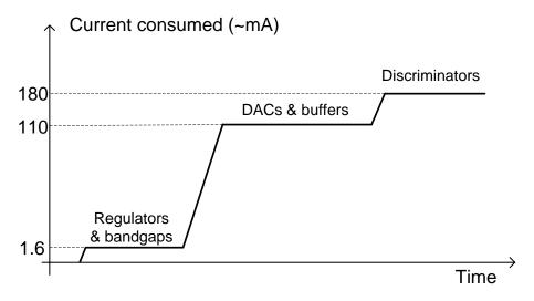
Figure 2.12: Current consumed by CPS during the startup.
