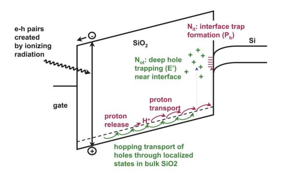
Figure 4.2: Band diagram of an MOS capacitor with a positive gate bias. Illustrated are the main processes for radiation-induced charge generation [2].
