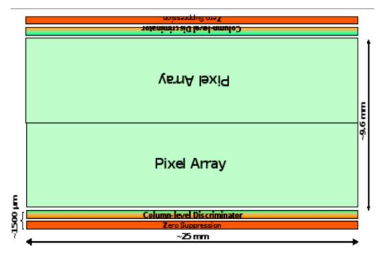
Figure 2.6: Diagram of two sided readout.
