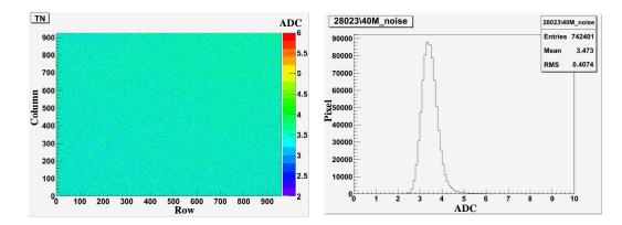
**Figure 5.19:** Distribution of the pixels noise in ULTIMATE at 40 MHz clock frequency (left) and Histogram of pixel noise in ADC unit (right) (1 ADC unit=4.15 e<sup>-</sup>) [28].
