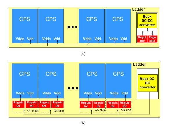
Figure 3.10: Schemes of the power distribution for CPS chips in a ladder: employing discrete regulators (Reg) (a) and on-chip regulators (Reg) (b).
