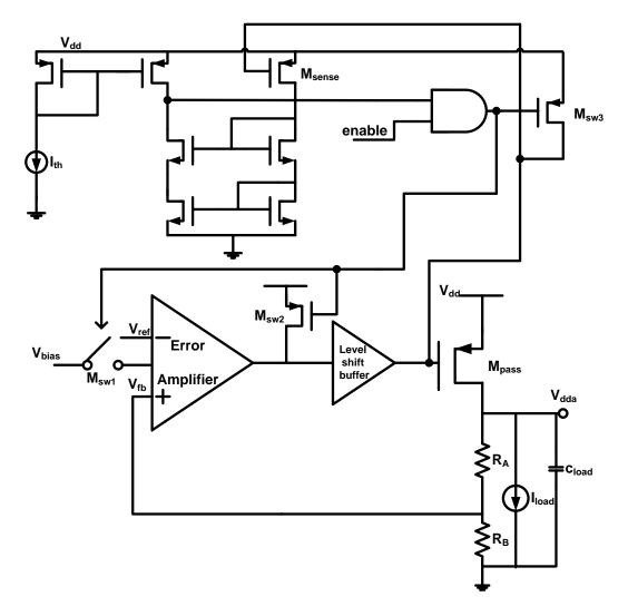
Figure 6.14: Implementation of the current limiter.
