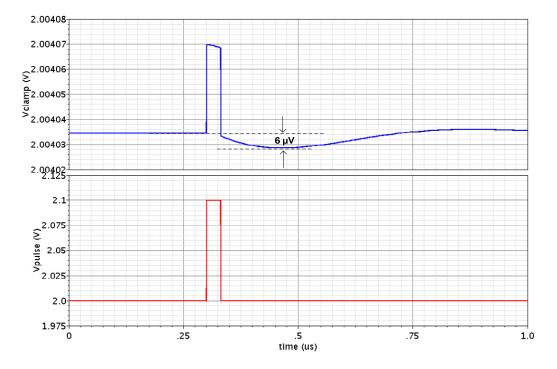
Figure 5.15: Simulated output voltage during the clamping operation.
