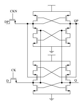
Figure 4.12: Improved SEU immune RAM cell (Whitaker cell) [29].
