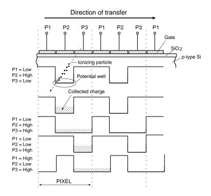
Figure 1.9: Structure of CCD and the operation timing.
