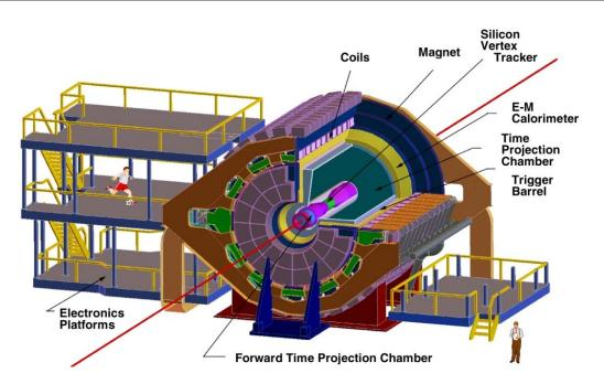
Figure 1.7: The layout of STAR detector and the cutting view showing the inner detector [6].
