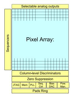
Figure 2.1: Structure of current CPS chip.
