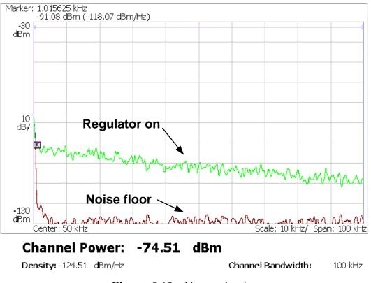
Figure 6.12: Measured noise.
