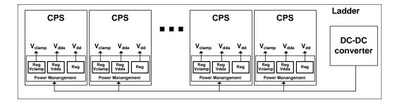
Figure 3.11: Power distribution for CPS in a ladder.
