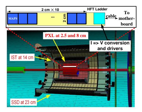
Figure 2.9: Diagram of the HFT and one ladder.
