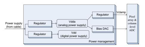
Figure 2.10: Block diagram of power management in CPS.
