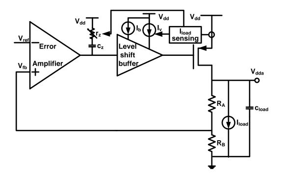
Figure 6.1: Block diagram of RegVdda.
