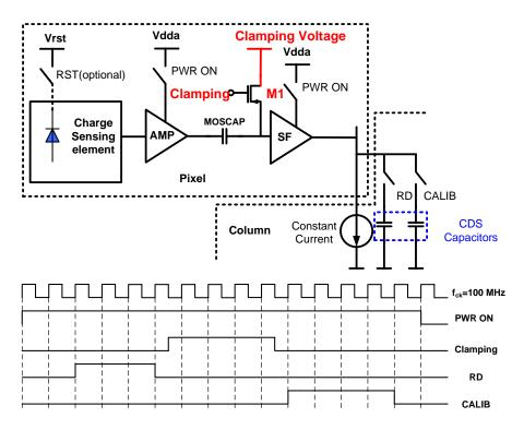
Figure 2.4: Block diagram and timing of CDS operation [14].
