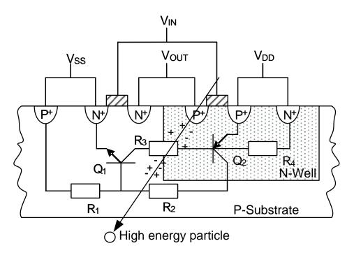
Figure 4.7: Principle of SEL in an inverter illustrating charges induced by a single high energy particle.
