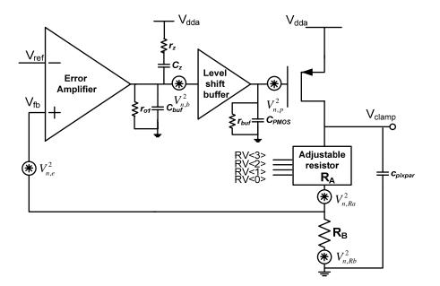
Figure 5.7: The block diagram of the proposed regulator depicting the equivalent resistors and capacitors of each stage and the main noise sources.
