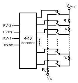
Figure 5.10: The digitally adjustable resistor  $R_A$ .
