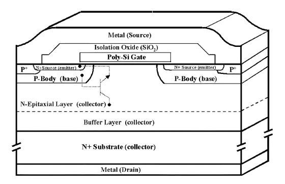
Figure 4.8: Cross section of n-channel power MOSFET [17].
