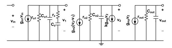
Figure 6.3: Equivalent small-signal model of the proposed regulator (open-loop).
