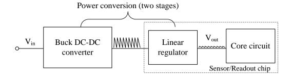
Figure 3.6: Post-regulator built-in the low-noise electronics.
