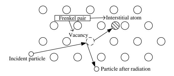
Figure 4.9: Atom displacement damage.
