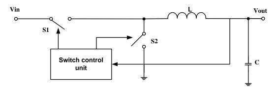
Figure 3.4: Architecture of buck converter.
