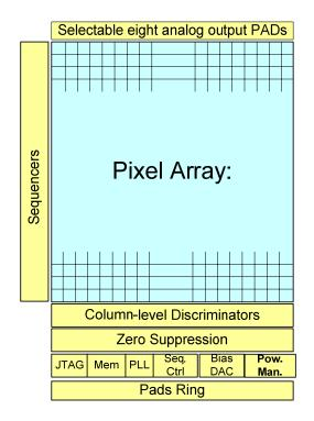
Figure 1.11: Structure of CPS chip.
