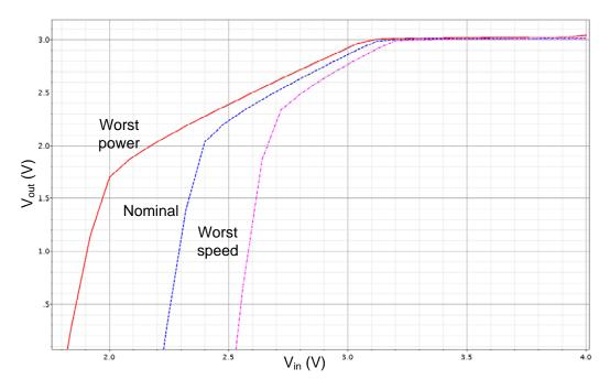
Figure 6.16: Simulated results of  $V_{dda}$  versus  $V_{dd}$ .
