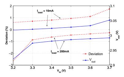
Figure 6.7: Measured line and load regulation.
