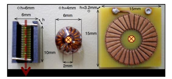
Figure 3.5: Solenoid (left), air core toroid (center), PCB toroid (right) [8].
