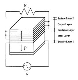
Figure 3.8: Piezoelectric transformer construction [16].
