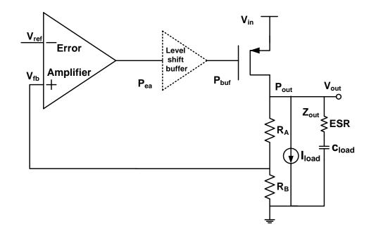
Figure 5.1: Block diagram of traditional linear regulator with buffer depicting the main poles and zeros.
