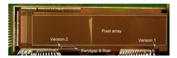
Figure 5.11: Microphotograph of the MIMOSA22-HRE chip.
