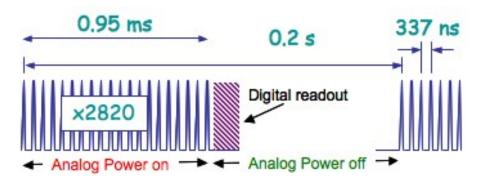
Figure 2.11: Power cycling options of ILC bunch timing [22].
