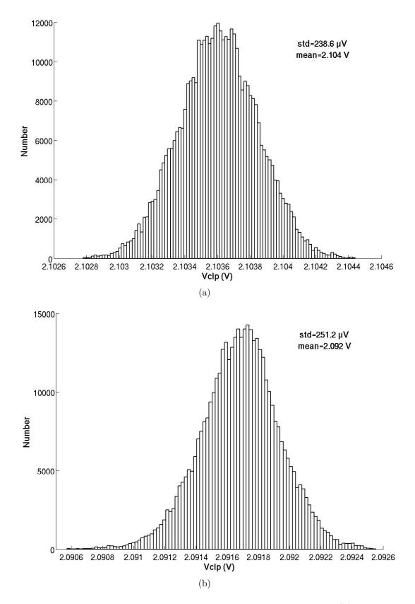
Figure 5.16: Histograms of the clamping voltage refer to version 1 (a) and version 2 (b)
