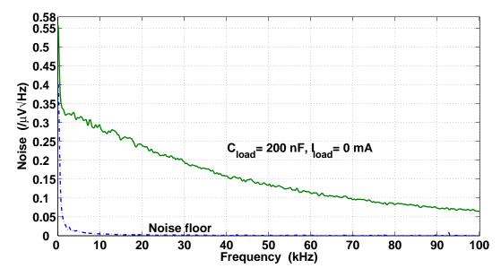
Figure 6.13: Measured output noise spectrum density.
