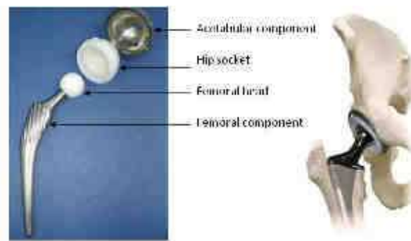
Figure II-12: Components of a total hip replacement [13]
