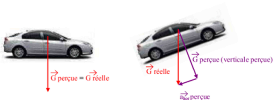
Figure 1.23: Principe du tilt-coordination (source : Vaillau 2010)
