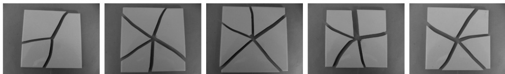
Figure 5.17 – Pictures of the tiles broken on the fitted test. In this condition, the variance on the number of cracks seems to be lower than the previous condition. On the first picture, 5 cracks propagated, but only 3 of them crossed the tile.
