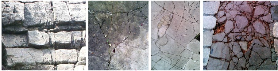
Figure 1.6 – Examples of naturally observable fractures due to aging processes.
