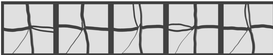
Figure 5.23 – Results of the simulation of the ceramic tiles. Star patterns that are observed in real experiments appear on the simulated tiles.
