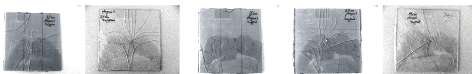
Figure 5.18 – Experiment on glass slabs - 4 punctual contacts. The results obtained are various and hard to interpret. Some noise may bias the experiments.
