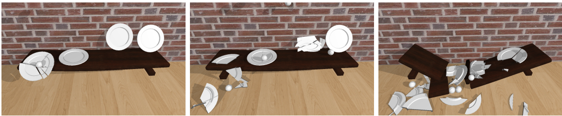
Figure 4.10 – Interactive smashing of plates. The user drops balls in real-time to smash the plates, and at the end of the simulation the scene consists of more than 45K triangles. The complete simulation runs at 8ms per time step on average, with a maximum of 17ms.
