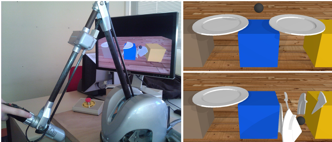
Figure 5.8 – Setup of the experiment. Left : photograph of the experimental conditions. The haptic interface is linked to the ball in the simulation, and the user can break the plates with force feedback. Right : screenshots of the simulation during a trial at the initial condition (top) and after one plate has been broken (right).
