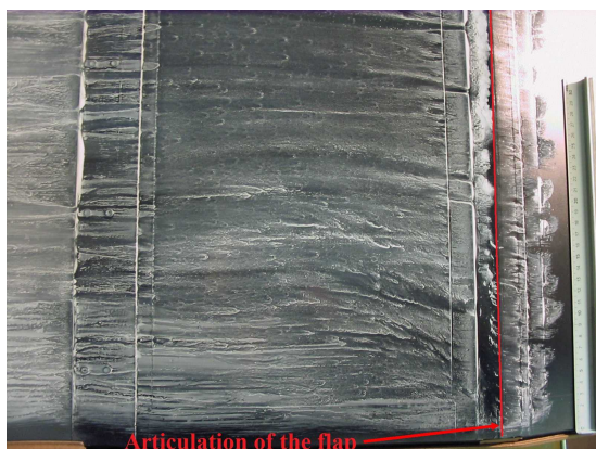
Figure 3.3: a) Oil film result on the center of the flap b) Oil film result near z = -1000 mm on the flap c) Oil film result near z = +1000 mm on the flap. \alpha = -2^\circ , \beta = -22^\circ and U_\infty = 10 m/s.
