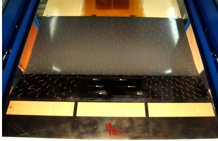
Figure 4. Example of wool tufts visualisation with control and no separation, \alpha = -2^\circ , \beta = -22^\circ and U_\infty = 10 m/s.
