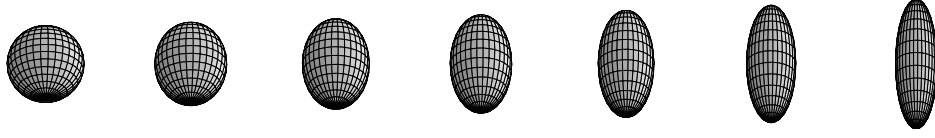
Figure 3.10: Diffusion tensors, represented as ellipsoids, for FA ranging from 0.0 to 0.6. The Mean Diffusivity is constant across the tensors.
