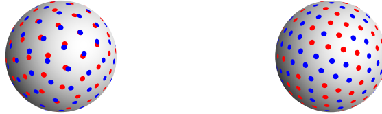
Figure 8.2: Extremal values of the weighting factor \alpha : minimum energy configurations for S = 2 shells, K_1 = K_2 = 50 points per shell, points reprojected on the unit sphere. (left) \alpha = 0 : all the importance is given to the uniformity of the configuration on each shell, independently of the other. As a result, the global coverage is non-uniform. (right) \alpha = 1 : the global angular coverage is uniform, but if we consider the repartition of points on shell 1 (blue dots) or shell 2 (red dots) separately, the angular coverage is not uniform.
