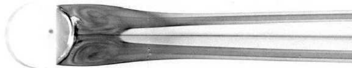
Figure 1.6: Streaklines showing a bifid wake. The plane of symmetry is imposed by the holding; Re = 250 . Przada et al. (2008).
