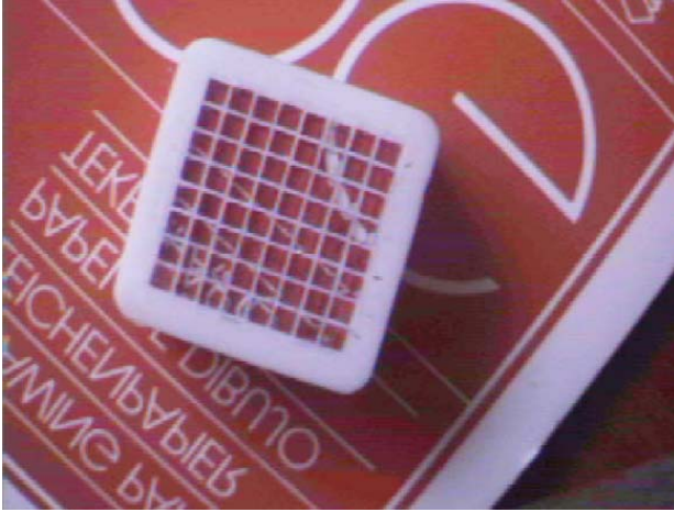
Fig. 2. Matrix made of Teflon and filled with LSO pixels. Distance between the crystals is 300 \mu\text{m} .
