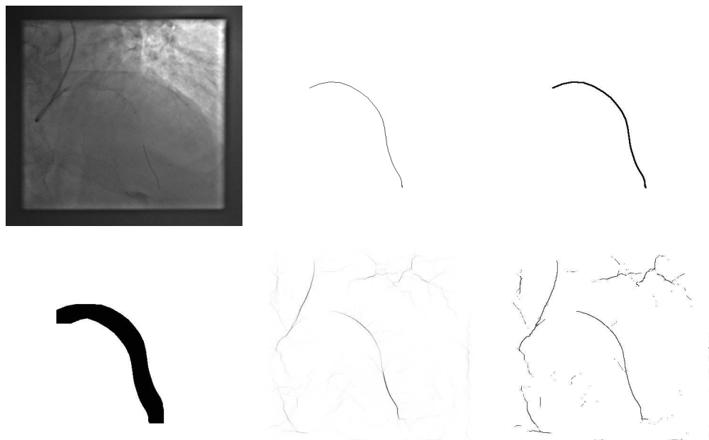
FIGURE 5.4: Illustration of the computation of TP, FP, TN and FN. Top row: original image, ground truth and dilated ground truth. Bottom row, ROI, output of our line enhancement technique and threshold and skeletonization of this output.
