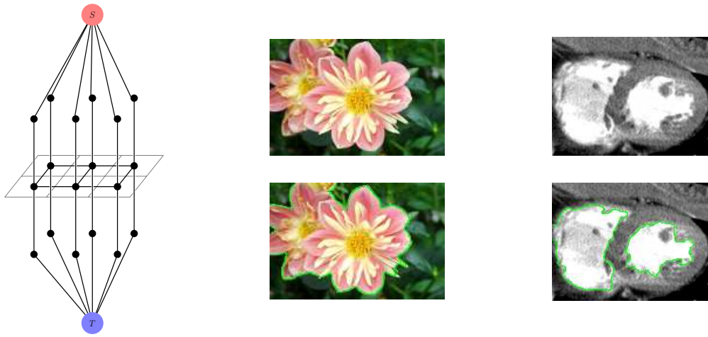
Figure 2.9: Example of graph construction to incorporate unary terms for unsupervised segmentation.
