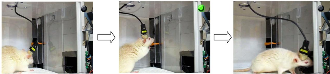
Figure 6.14 The close-loop real-time stage of the experiment. The rat presses the pedal but decision whether to give a reward is made on the basis of the ECoG signal.
