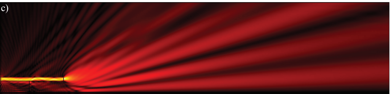
Fig.5-6. Numerical simulations to compare emission from the edge of a PMMA waveguide on a planar silica substrate (a) and on a substrate with a 3 \mu\text{m} underetch (b). c) Fringes generated by the emission reflection from the substrate in pedestal configuration. Color gradient represents the z-component of the electric field, E_z [V/m].
