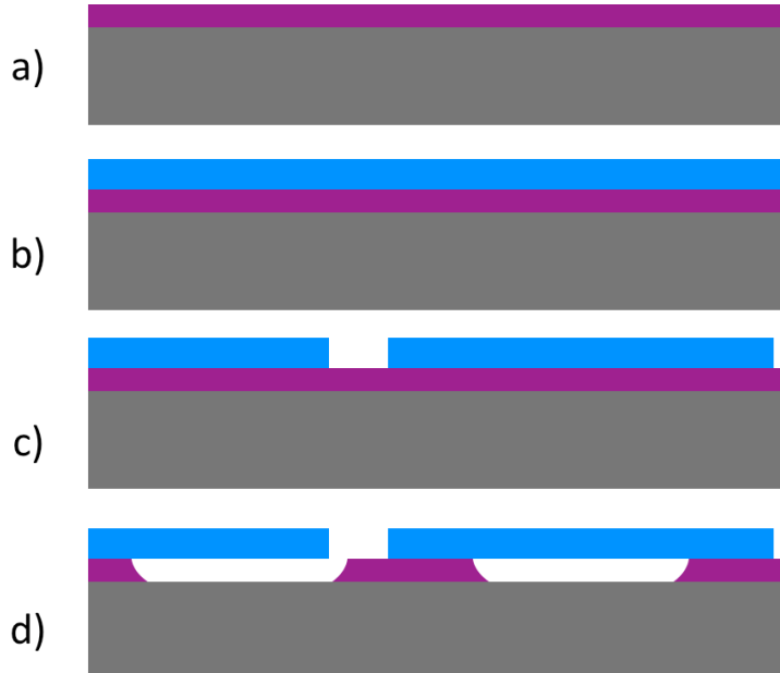
Fig. 4.14: Process for fabrication of \text{SiO}_2 beams (single-clamped cantilevers or clamped-clamped beams): a) an amorphous silicon layer is deposited on a silicon substrate; b) growth of a low-stress \text{SiO}_2 layer using PECVD; c) lithography and etching of beams; d) release of the beams by isotropic \text{XeF}_2 etching.
