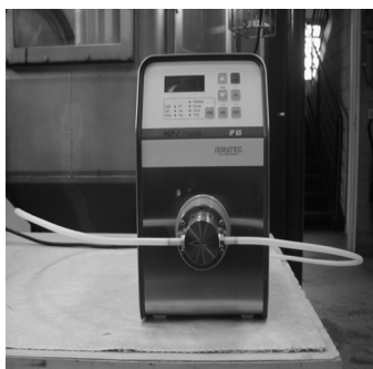
Figure III.21. Pompe à engrenage.
