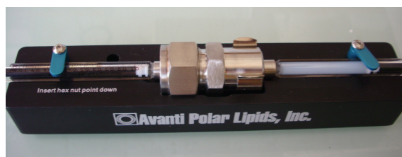
Figure 3.4: The Avanti® Mini-Extruder to obtain large unilamellar vesicles.
