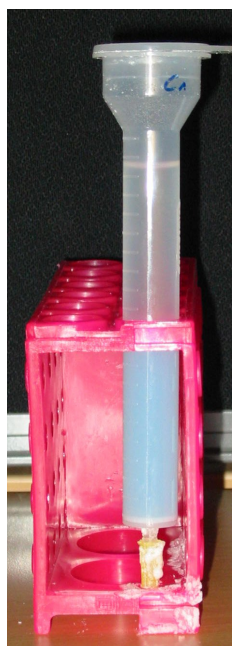
Figure 3.2: Picture of a Ni-NTA agarose (QIAGEN) column used for nickel affinity chromatography to purify MBP and P2 proteins. Protein-buffer-solutions are loaded onto a column with 10 ml of Ni-NTA matrix and the buffer can flow through the closable hole on the bottom (yellow seal).
