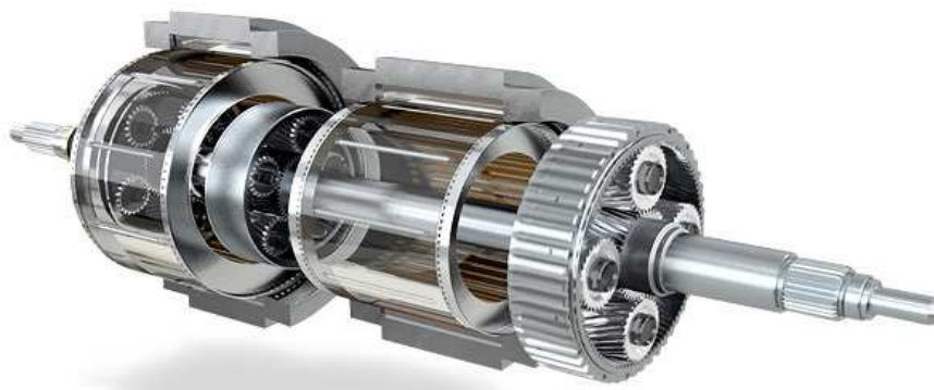
Figure 2 – BMW X6 Active Hybrid with three planetary gear sets [2-3]
