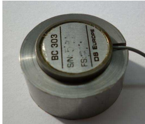
Figure 3.25: Metal cover in which is placed the force sensor
