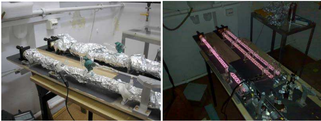
Fig. 4.12. Cleaning process of the OP cells. Left: A heating tape ( 100^{\circ}\text{C} ) was wired around each cell while a vacuum was produced by a TMP. The aluminium foil visible on the picture keeps the heat close to the glass. Right: Plasma discharge with 20 mbar of ^4\text{He} . The shape of the plasma is made of rings close to each electrode.
