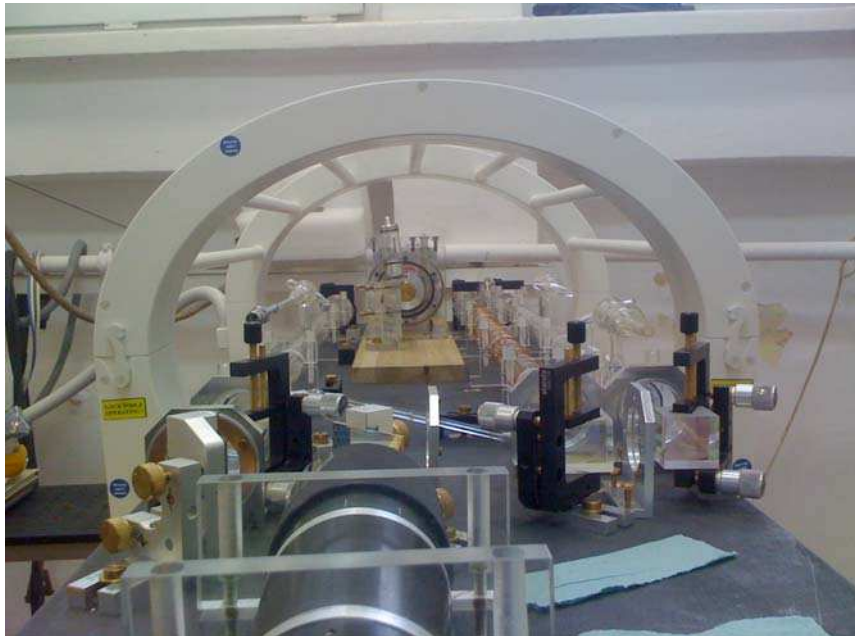
Fig. 4.11. Picture of the OP plate of the high field polarizer during construction. On the foreground, the pair of axicons is mounted on Plexiglas holders. Non magnetic holders were ordered for mirrors, half and quarter-wave plates and polarizing beam splitter. The peristaltic compressor can be seen on the background. All the system fits inside the birdcage coil.
