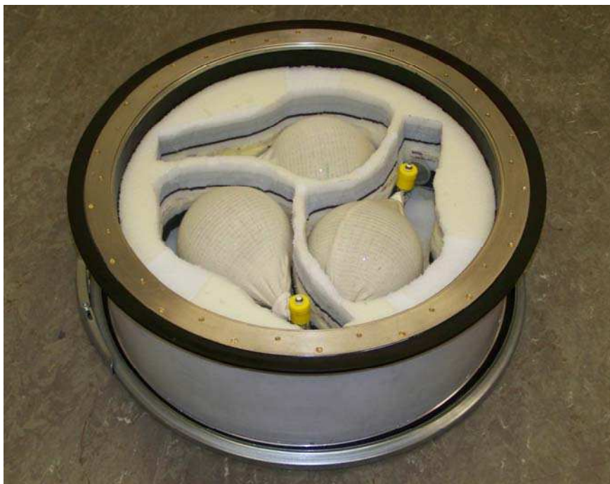
Fig. 2.5. Transport box and vessels from Mainz University group for ^3\text{He} storage during journey to hospital.
