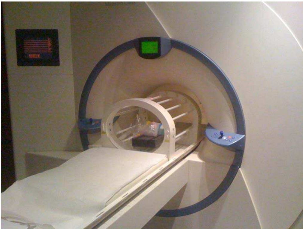
Fig. 2.10. Sonata scanner in John Paul 2 nd Hospital with 3 He coil from RAPID Biomedical. In the center of the coil, a first phantom (see text) is placed for angle calibration experiment.
