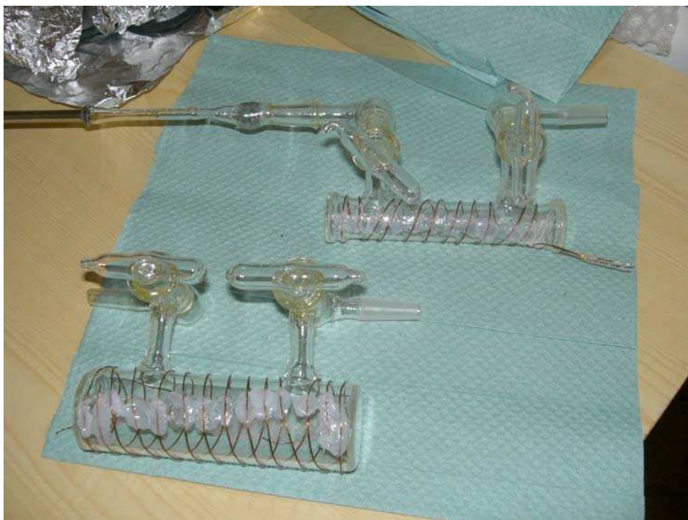
Fig. 4.1. Picture of two open cells used for preliminary tests inside our superconducting magnet at 1.5 T. The first cell at the bottom of the figure has a cylindrical shape (diameter: 34 mm) whereas the top one has a bone-shape (diameter: 16 mm) and is connected through a glass-metal connection to a turbomolecular pump for cleaning purpose.
