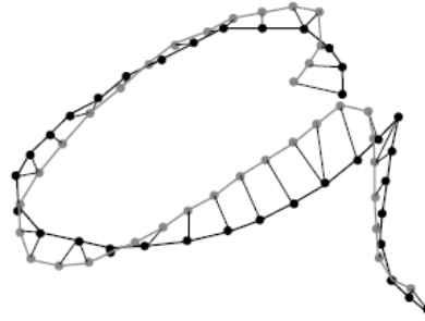
Figure 2.1: The point-to-point correspondence of two characters established with a DTW-algorithm [1]
