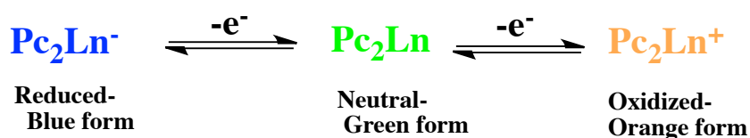
Figure 3.21 Neutral, oxidized, and reduced forms of Ln(Pc) 2
