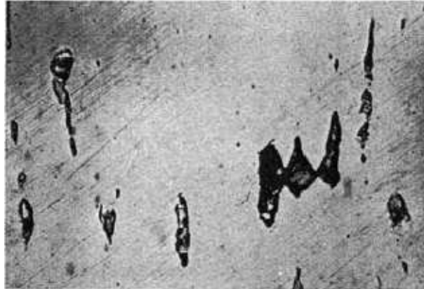
Figure 4.1: Internal necking in the central region of an as-rolled copper tensile specimen. \times 300 [Putt 59].
