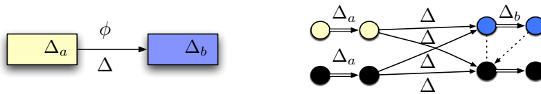
Figure 7.6: The encoding of two temporal objects a and b . The time conditional relations representing its duration and a time conditional relations express precedence between a and b with a condition \phi . Mutual conflicts are represented by a dashed line. Black-colored events have invisible actions.
