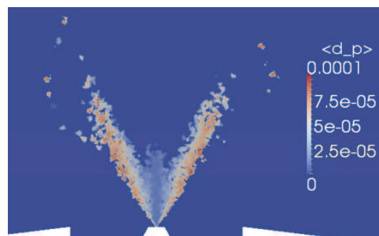
Figure 4.14: Mean instantaneous droplet diameter, showing the flame structure when the spray injection follows approach (B).
