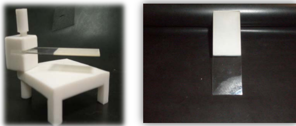
Figure 2.11. \text{N-F} codoped \text{TiO}_2 prepared by sol-gel solvothermal method
