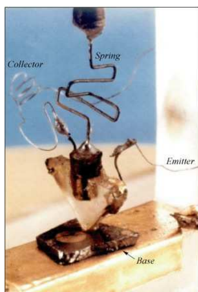
Fig.1.1. The first point contact transistor. John Bardeen , Walter Brattain and William Shockley , Bell laboratories, Murray hill, New Jersey, 1947.
