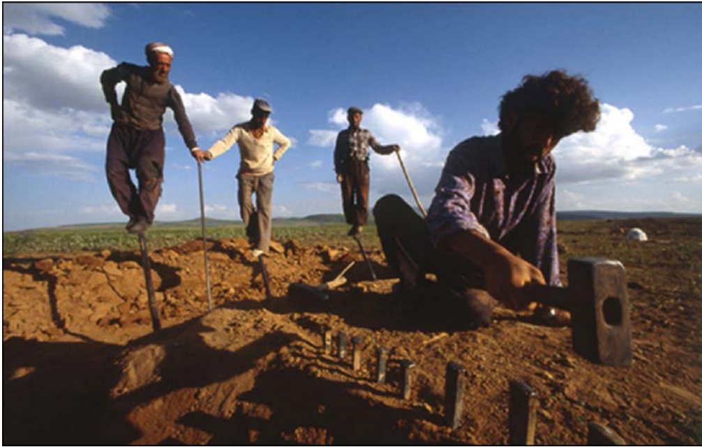
Figure 2.17. Traditional mining of ignimbrite blocks, near Yasin hill at west of Ahlat town. Photograph by Adem SÖNMEZ ( Those who wrest a living from the stone ), used with permission of photographer.
