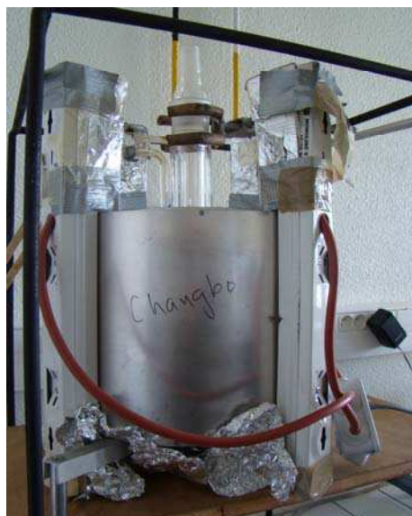
Figure III-C-3 Home-made photoreactor with four tubes (Philips TLD 15W / 05)
